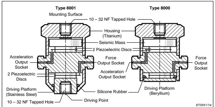
Fig 2 Schematic drawings of Types 8000 and 8001
