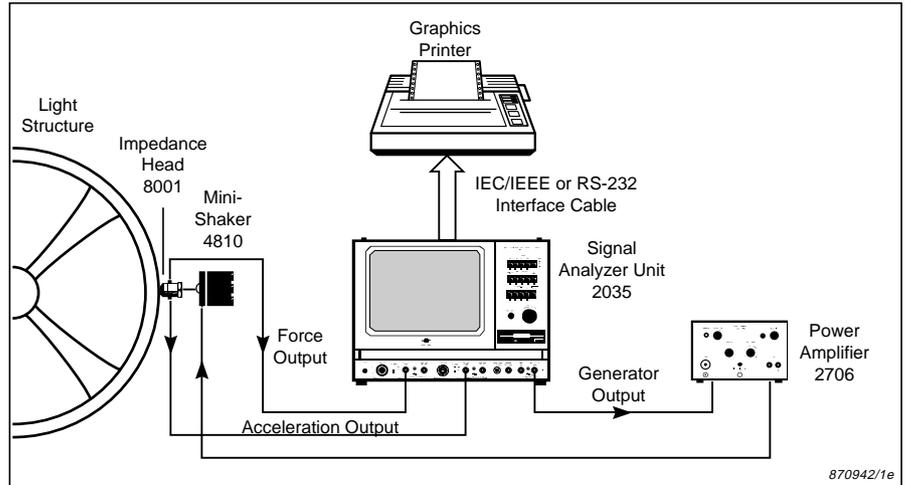
Fig. 3 Set-up for mechanical impedance and mobility measurements
