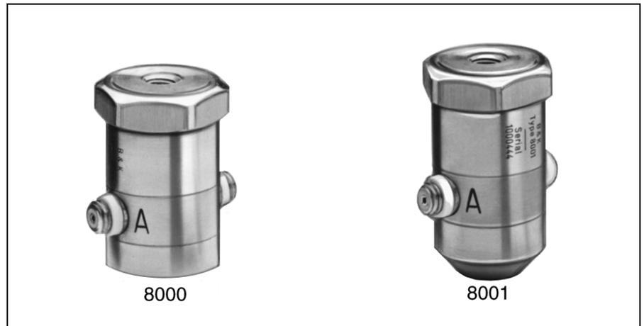
Impedance Heads Types 8000 and 8001 offer a way to measure the applied force and response at a point on a light structure. Simultaneous measurement of both of these quantities can provide data on the mechanical mobility and impedance of the structure at the point of interest. These measurements form the starting point of investigations into other dynamic properties such as acceleration, compliance, damping, loss factors and resonance frequencies.
